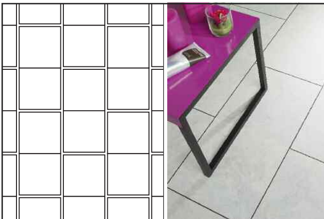
Square tile with strip around every 2 tiles, laid brickwork (rectangular tile effect)
